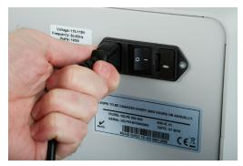
**a.** Unplug the Light Booth from the wall outlet, then remove the power cord from the rear of the unit.
