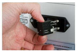
**b.** Using a flathead screwdriver, press the tab to remove the voltage selector insert.
