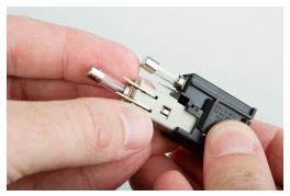
**d.** Reinsert the voltage selector, confirming that the proper voltage is now showing, and replace the voltage selector insert into the rear of the unit.
